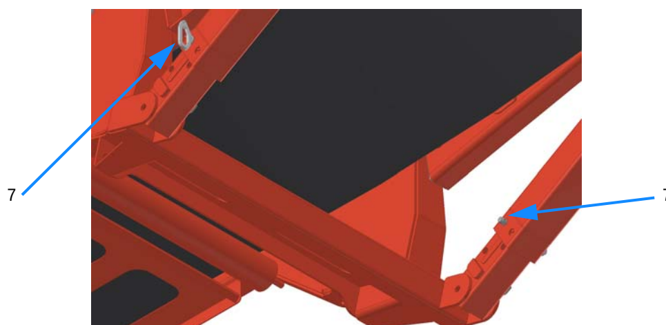
7: Move the supports to the correct position and install the locking pins. Three positions are available.
