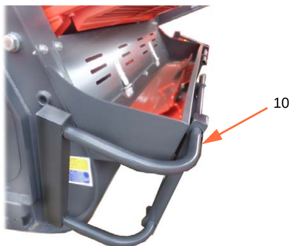
10: Remove handrail ends from transport position
