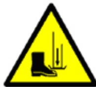
Crushing Hazard - Feet
