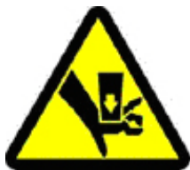
Crushing Hazard - Hands
